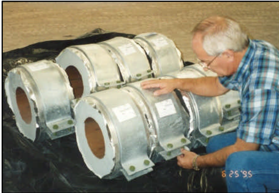
Hotshoes under inspection
