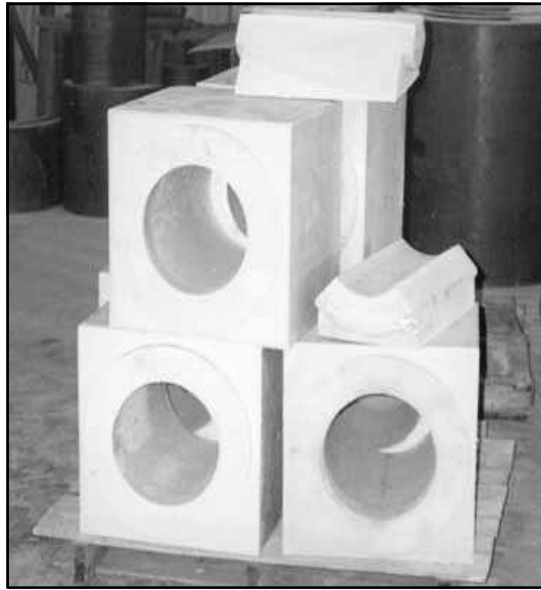
"Blanks" used in the fabrication of Resting Coldshoes
